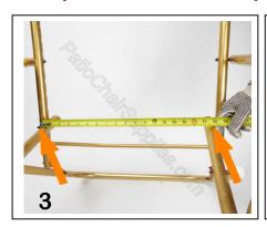
Place tape measure on the outside part of the frame (left side) and measure across to the outside part of the frame to the right side as shown in (Pic.3)
