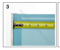
Towards the top part of the chair's sling, place the tape measure in the center of one rail and measure across to the opposite rail as shown in (Pic.3)
