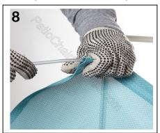
Slide the plastic splines into the sling pockets on both sides as shown in (Pic.8)
