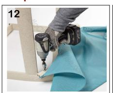
Use an impact drill to remove all the bolts (spacers or washers) that hold the rail of the side you inserted the sling as shown in (Pic.12)
