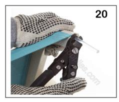
Cut all the excess spline as shown in (Pic.20)
