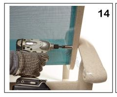
On the side that is still attached to the frame, loosen all bolts 3/4" of the way using an impact drill as shown in (Pic.14)
