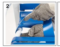
Push the rivet into both strap. Insert the rivet into the hole of one side of the chair frame and if necessary use a hammer to tap it in. as shown in (Pic.2)
