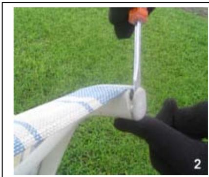
Using a flat head screw driver remove both end caps from the top of your chair and both end caps from the bottom of your chair. Be very careful when removing the end caps, they could be very dry and brittle since they are exposed to outdoor elements. Pic.2
